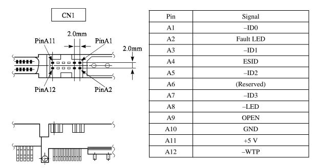
Figure 4.16 External operator panel connector (CN1)
